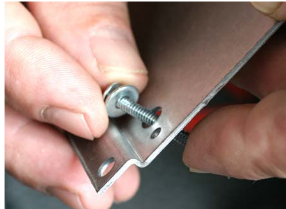
Figure 3: Use washers on the screws that attach the board to its mounting plate.
